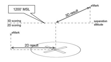
When goals/targets above the ground are used, results based on track points will be 3D-distance
